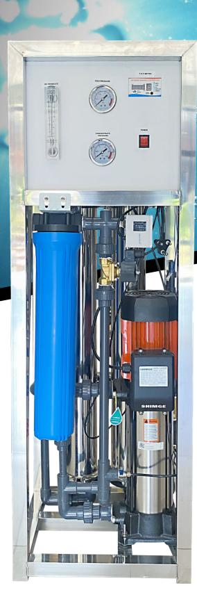
**Puritech** compact commercial reverse osmosis system is a durable piece of equipment which, with proper care and maintenance will last for many years. ECO series systems are part of a family of reverse osmosis units designed for operation with fresh and brackish feedwaters having TDS values below 1,500ppm. Models are available with permeate outputs of between 150 and 1,000 litres/hr as shown in the specifications.
