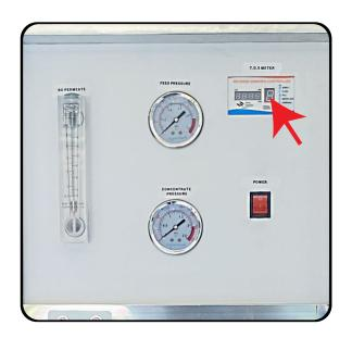
when the red power button is pressed it means that there is now power to the RO system, the ROC (Reverse Osmosis Controller) displays/ flashes9 number 8 (please see picture below) and thereafter continues its flushing cycle/s for about 60-90 seconds, this is indicative that the RO system is running correctly.
