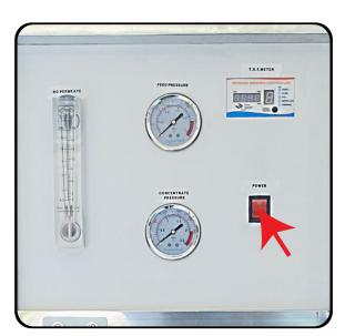
Once the membrane/s are inserted, the next step is to run the RO system, by pressing the red power button, see red arrow for reference above:
