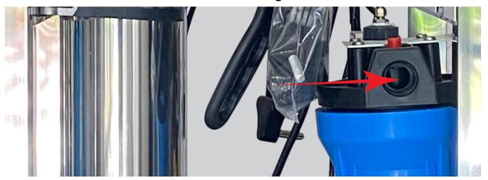
Feed water inlet connection from the 20" blue filter inlet solenoid i.e., the arrow in red above:
